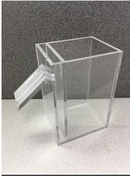
Figure 3-7(a). Example of a Displacement Vessel.
