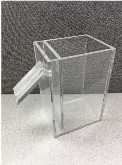
24 Figure 3-7(a). Example of a Displacement Vessel.
